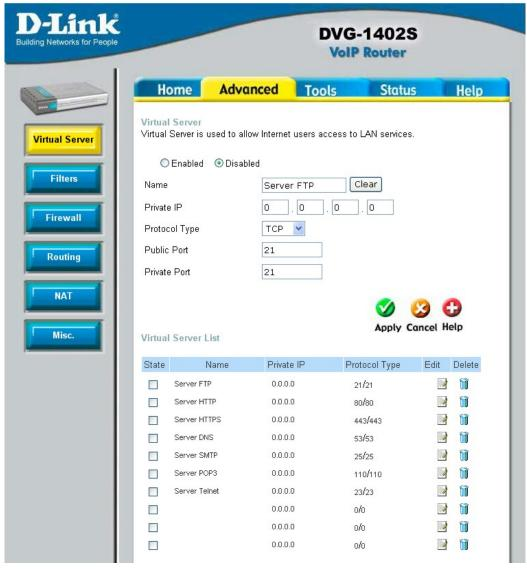
To view the following window, click on the **Advanced** tab at the top of the window and then click the **Virtual Server** button to the left. The **Virtual Server** will allow remote users access to various services outside of their LAN through a public IP address, such as FTP (File Transfer Protocol) or HTTPS (Secure Web). After configuring the Router for these features, the Router will redirect these external services to an appropriate server on the user's LAN.
